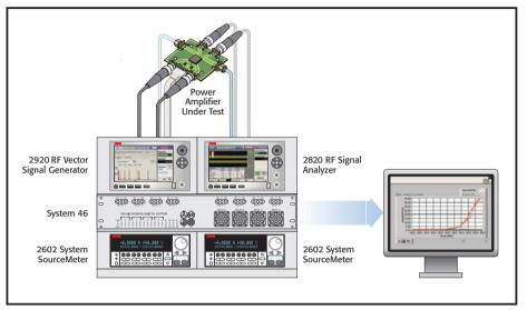
Through the use of test script control and intra-instrument triggering, this Model 2920-based RF power amplifier test system can reduce test times by up to 70%.
