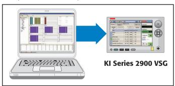
Create waveform files off-line on a PC with Keithley's free SignalMeister waveform creation software, then download them to the ARB memory of any Keithley Series 2900 RF Vector Signal Generator.
