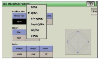
The Model 2920-DIG Flexible Digital Modulation option simplifies controlling a test signal's modulation format, symbol type, filter, data pattern, and data length.
