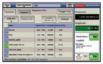
The Model 2920-ARB-xx Arbitrary Waveform Generator option provides 100 megasamples (100Msa) of memory for storage of large waveforms or multiple waveforms, with up to 80MHz signal bandwidth.
