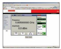
A built-in LXI webpage interface allows monitoring and controlling the Model 2920 from any Internet connection anywhere in the world.
