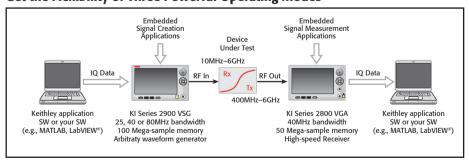
Keithley's Series 2900 RF Vector Signal Generators and Series 2800 RF Vector Signal Analyzers are engineered for operating versatility. Use built-in applications or download I-Q waveform data from a connected PC and upload signal waveforms.
