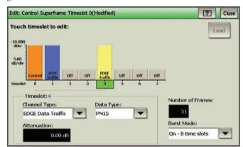
Use the Model 2920-GSM option's waveform edit menu to select the channel type and data type for each time slot.
