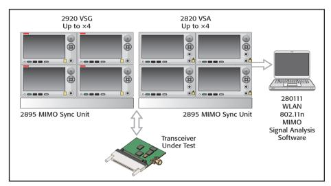
This  $4\times4$  MIMO test system ensures precise synchronization and low jitter when testing WiFi, WiMAX, and other MIMO devices and equipment.
