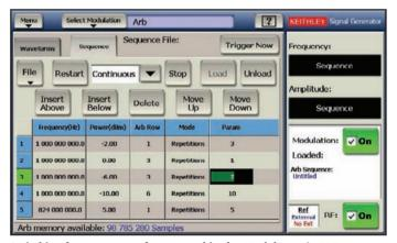
Switching from one waveform stored in the Model 2920's ARB memory to another takes just 3ms under GPIB control or is instantaneous when in the ARB Sequence mode. Here, the waveform sampler moves from the last point of an ARB waveform to the first point of the next waveform within a single clock cycle. The ARB waveforms can be "played" in any order or pattern desired, providing added flexibility for measurement speed enhancement.
